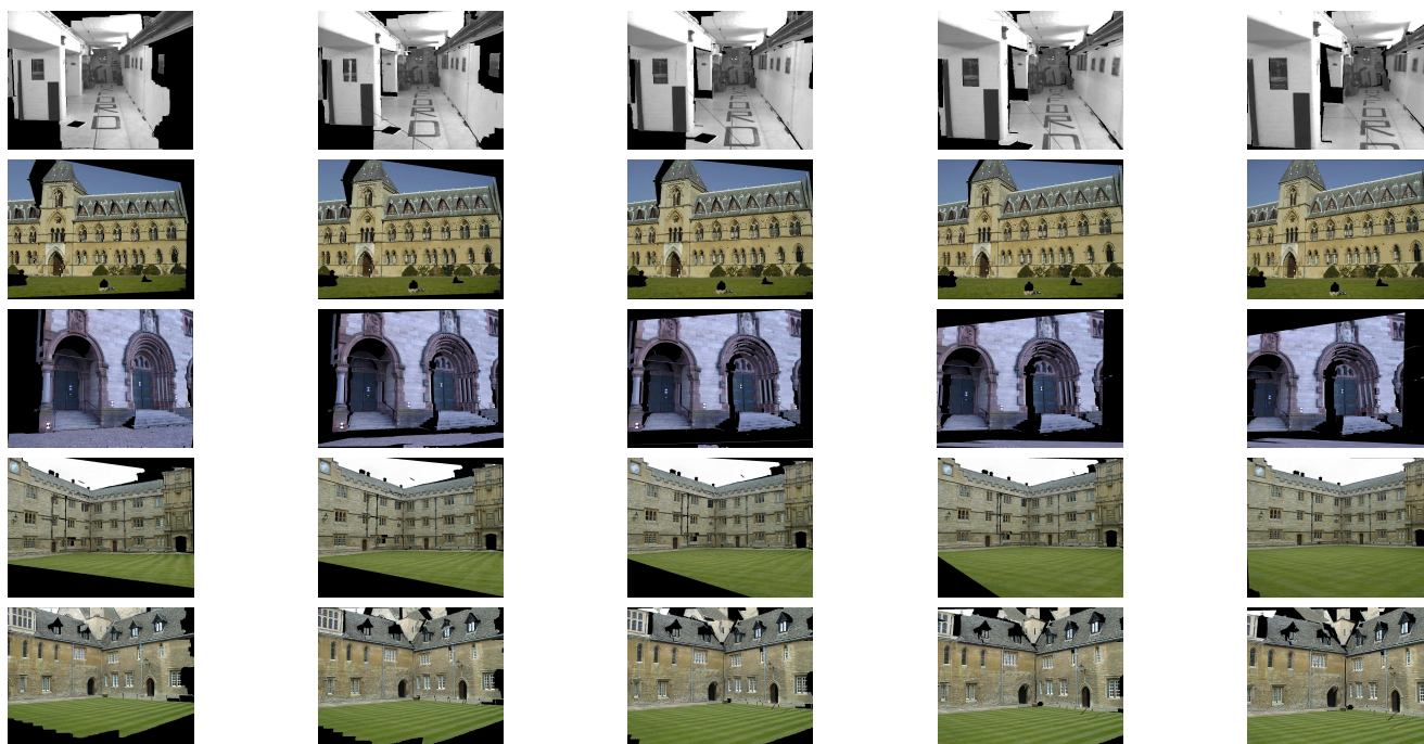
Figure 3: Projection of the textured piecewise-planar approximation of the scene's 3D on virtual views in-between the two cameras of the wide-baseline stereo pair.
